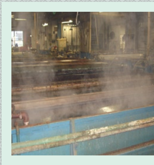
A row of plating tanks with fuming contents. Amazingly, the room has little odor; its air is much more breathable than the average printing plant.
