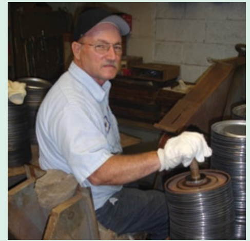
Wayne Shelly, Chief Polisher. This man, a star in a proud dwindling profession, is the very heart of the plating process at Jamestown Electro Plating. He is surrounded by stacks of shaped disks that — when polished and plated — will serve on the ceilings of trucks and busses as bases for lighting fixtures.
