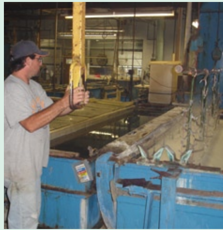
Plater/Operator Brian Watson raises a rack filled with parts that have just been plated.
